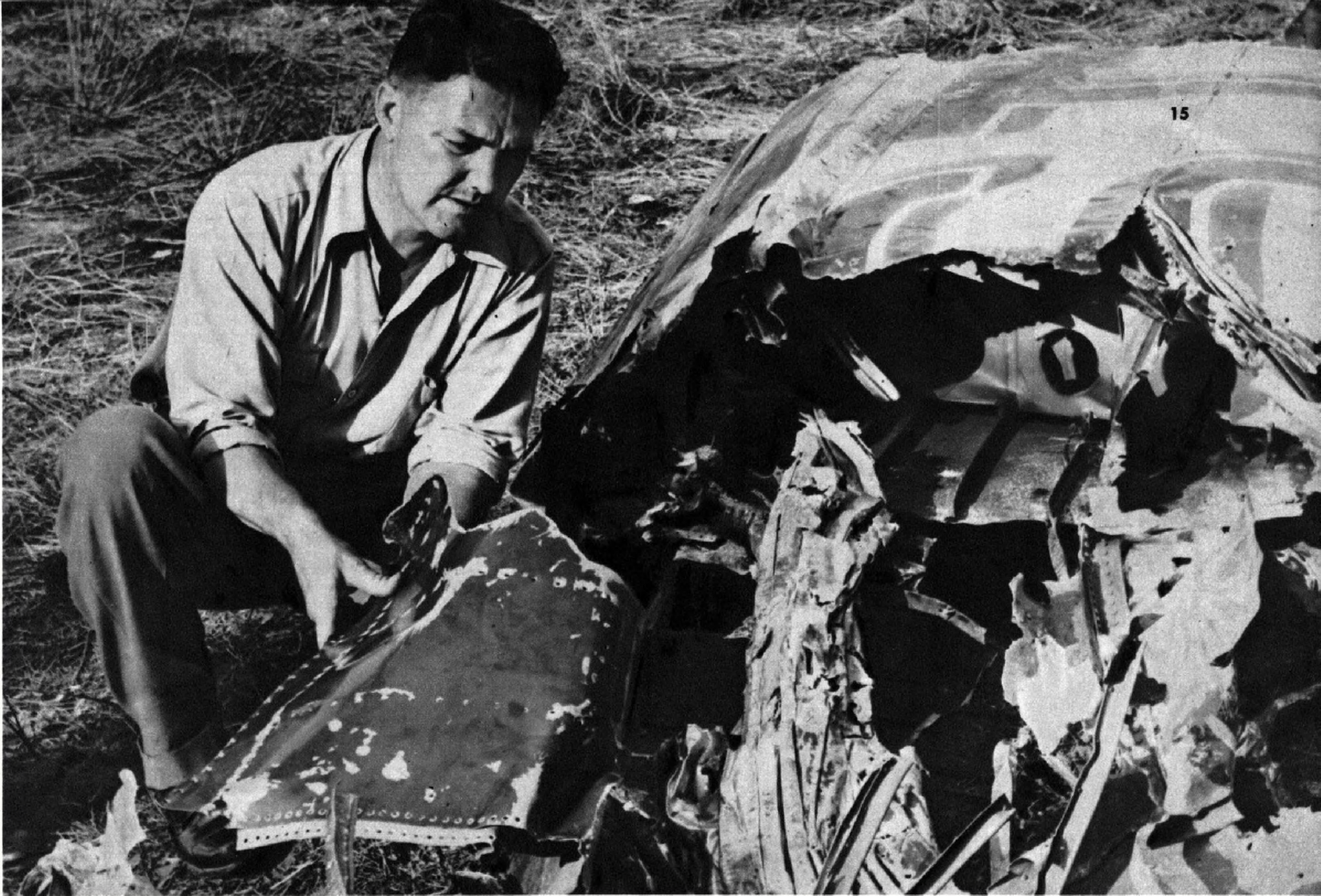
CAB investigator Joseph Fluet matching wing sections to determine initial contact point of a transport and an F6F that collided in mid-air
